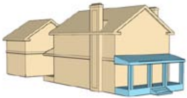
F SHED ROOF PORCH
