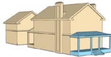
C HIPPED ROOF PORCH
